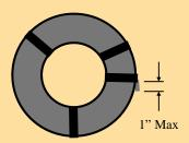
At least one band attached within 1-inch from end (or belly band).
