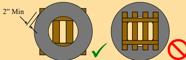
Outside boards extend beyond coil OD at least 2" each corner, supporting the coil on 4 corners. Skid diagonal greater than coil OD by at least 4".
