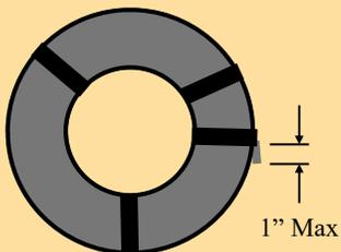
Four bands required with one band attached within 1-inch from end
