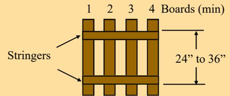
4 boards minimum, evenly spaced. 2 stringers parallel and 24" to 36" apart, outside dimension. Skid construction solid, no nails protruding.
