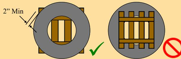
Outside boards extend beyond coil OD at least 2" each corner, supporting the coil on 4 corners. Skid diagonal greater than coil OD by at least 4".
