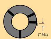
Four bands required with one band attached within 1" from end (or belly band)
